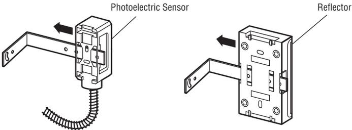
3. Attach mounting bracket to solid surface with hardware (not provided).
