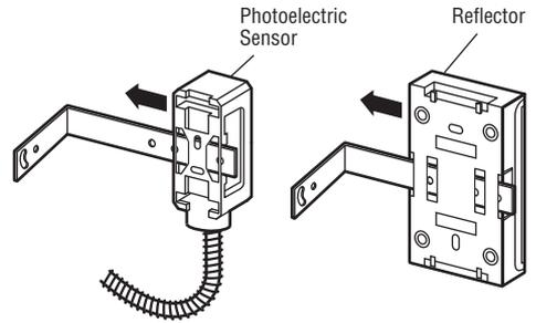
3. Attach mounting bracket to solid surface with hardware (not provided).
