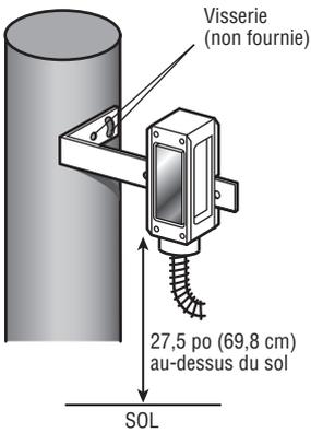
MONTAGE AU MUR AVEC SUPPORT (FOURNI)
