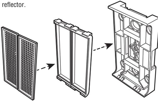
2. Slide the photoelectric sensor and the reflector onto the mounting brackets and secure with self-tapping screws provided.
